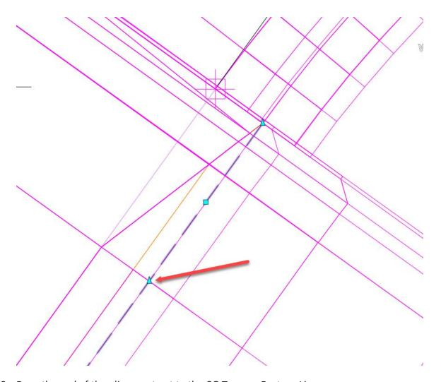
3. Drag the end of the alignment out to the CG Terrace Feature Line
