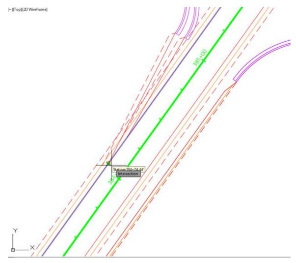
3. Next select where the main road alignment matches into the turn lane taper
